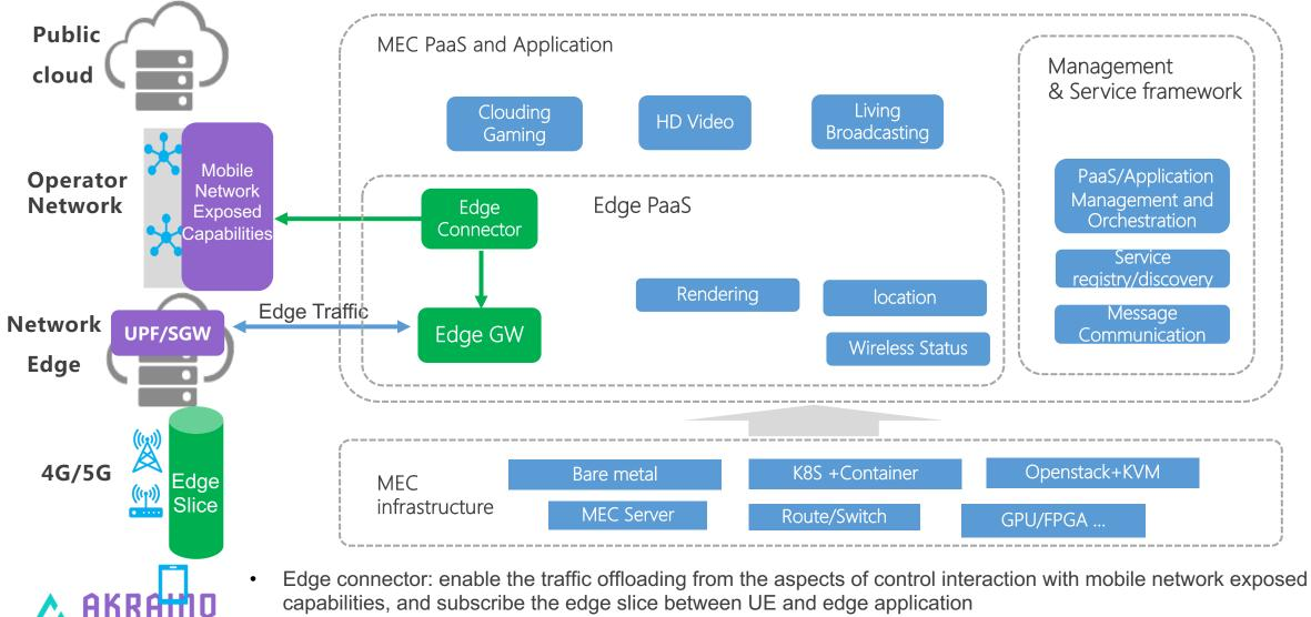
• Edge GW: enable the traffic offloading from the aspects of data plane with load balance, application proxy, traffic management, local traffic routing
