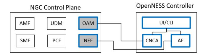
The following pictures show the microservice architectural view of the OpenNESS solution with 5G integration components:
