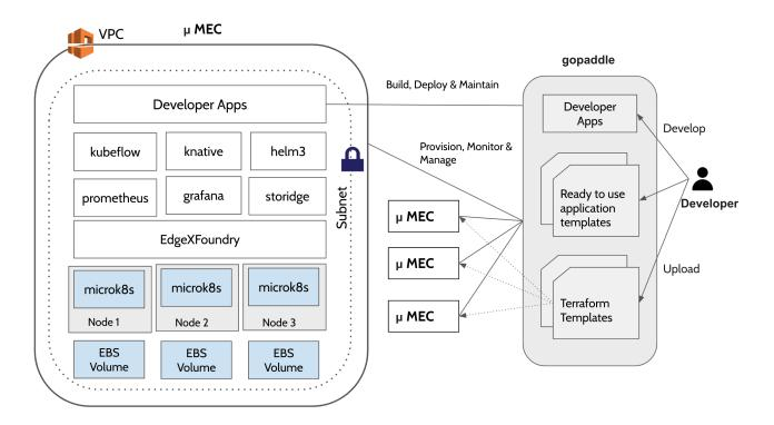
The blueprint consists of microk8s as the light weight Kubernetes distribution. Microk8s' zero-ops capability offers all the Kubernetes networking and storage configurations out of the box with built-in add ons for serverless (knative) and machine learning workloads (kubeflow) etc. Terraform is used to automate the installation and configuration of a multi-node microk8s cluster on AWS VPC.
