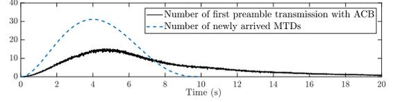
Fig. 2. Traffic spreading effect of ACB scheme with  $\{p_{ACB}; T_{ACB}\} = \{0.5; 4s\}$  for 30,000 devices arriving according to Beta(3,4) over 10 seconds
