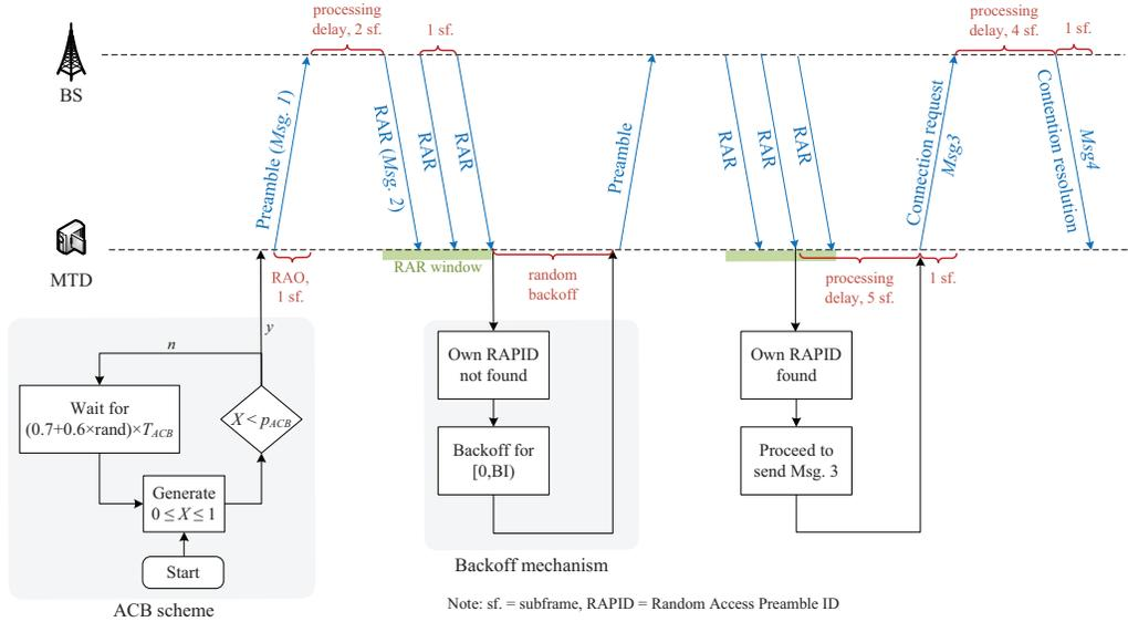
Fig. 1. LTE contention-based random access procedure with ACB activated
