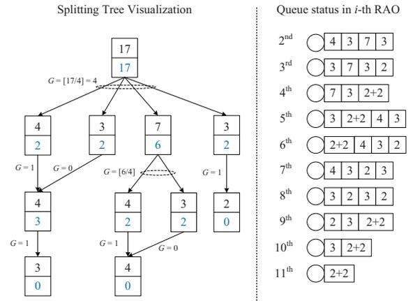
Fig. 4. Operation of proposed DQ-based contention resolution protocol,  $K = 4$
