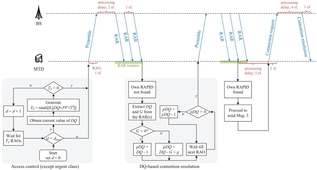
Fig. 5. Random access procedure for the DQ-based framework
