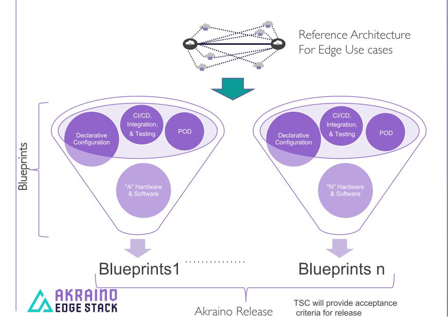
**Blueprints** — Approved and tested declarative configuration based on use cases, set of Hardware & Software, Point of delivery (POD).
