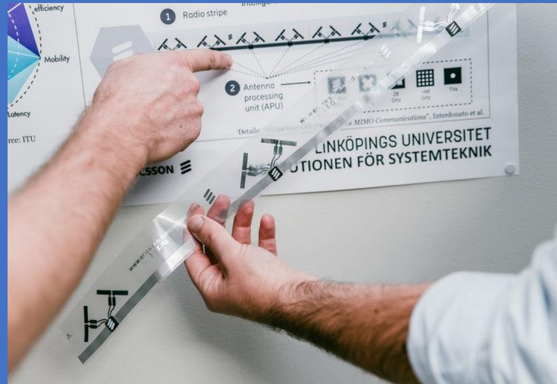
A piece of Ericsson's Radio Stripe networking tape reveals radio modules and the power and networking cables connecting them.
