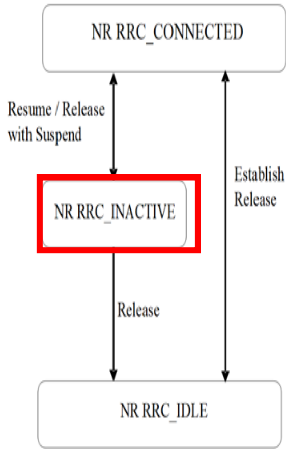
Figure 4.2.1-1: UE state machine and state transitions in NR
