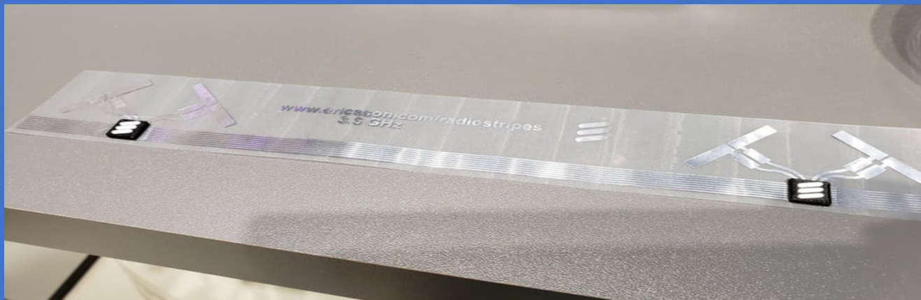
A piece of Ericsson's Radio Stripe networking tape reveals radio modules and the power and networking cables connecting them.
