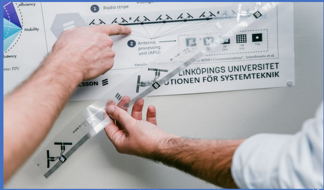
A piece of Ericsson's Radio Stripe networking tape reveals radio modules and the power and networking cables connecting them.
