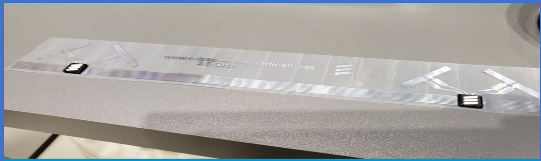
A piece of Ericsson's Radio Stripe networking tape reveals radio modules and the power and networking cables connecting them.
