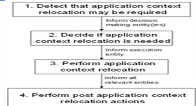
Fig. High level overview of ACR (Application Context Relocation)
