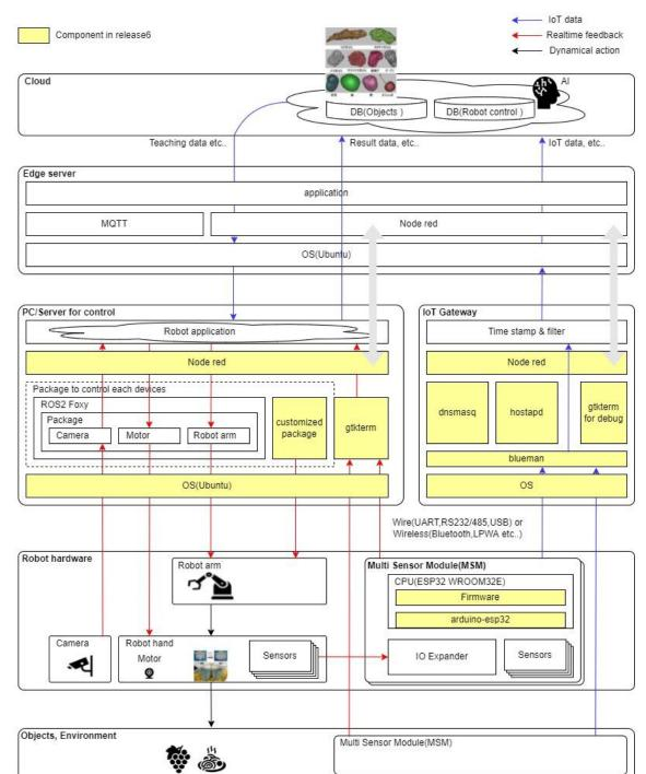
The following figure indicates platform and software architecture in release6.
