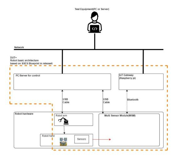
The following figure indicates HW and its connection.
