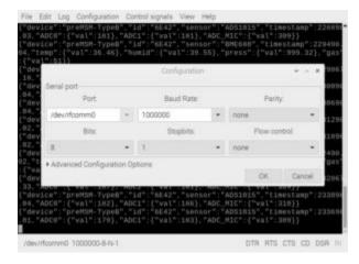
Enter the port according to the hardware configuration, such as /dev/rfcomm0 or /dev/rfcomm1. For the baud rate, enter 1000000 bps (1Mbps). Other than that, the defaults are OK.
