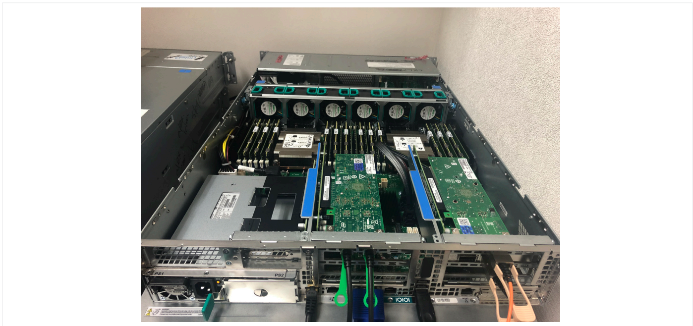
Figure 5. Photos of the Intel® Server Board S2600WFT 2RU commercial off-the-shelf DUT
