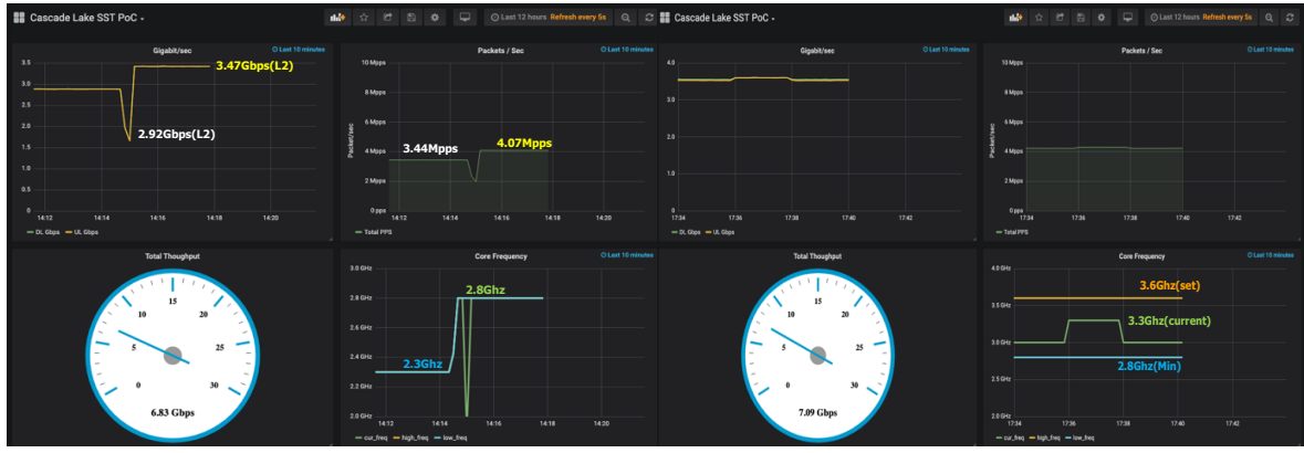
Figure 6. Throughput improvement from 2.3 GHz, 2.8 GHz, and 3.3 GHz
