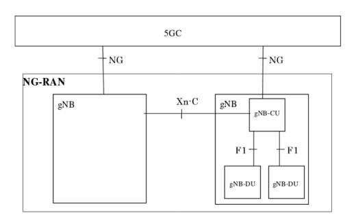
The DU (Distributed Unit) / CU (Centralized Unit) split enables running the CU in an edge cloud
