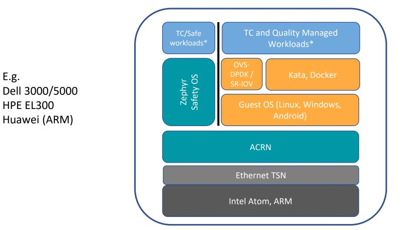
Virtualized, Functionally Safe workloads in addition to others Easily Extensible and Expandable, by just adding more systems Evaluating Airship for ZTP and deployment \* See next page for some sample targets
