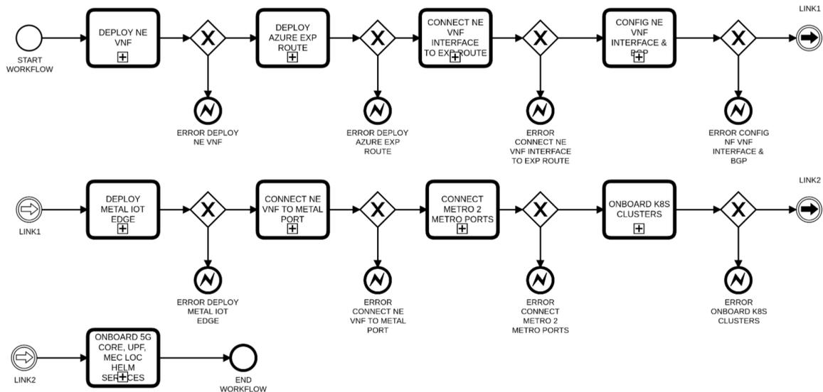
The end to end infra orchestration Camunda workflow steps to demonstrate Public Cloud Azure, Equinix Network Edge and Metal IoT k8s cluster Infrastructure orchestration:
