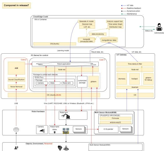
The following figure indicates platform and software architecture in release7.
