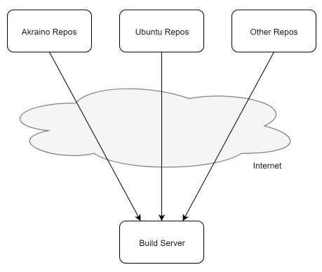
The 'Build Server' is only used to build and deploy a Regional Controller (RC). Therefore it can be considered ephemeral to the deployment and operation of the other Network Cloud RCs and Unicycle/Rover edge pod infrastructure.
