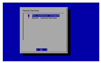
Arrow down to and press the spacebar to select the network interface to be used for the external network.
