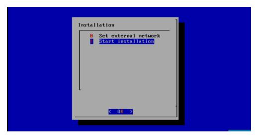
After selecting **Start Installation**, the installation should start automatically, and the content of /srv/deployment/log/bootstrap.log should be displayed on the remote console.
