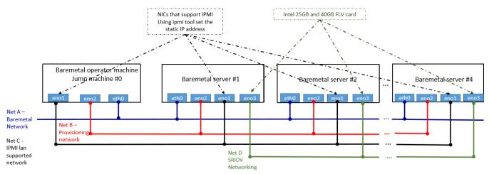
Net A – Baremetal Network, lab networking for SSH, It is used as the control plane for Kubernetes, used by OVN and Flannel for the overlay networking with Internet access
