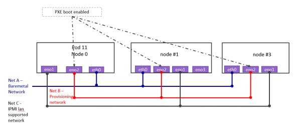
Net A – Baremetal Network, lab networking for SSH, It is used as the control plane for Kubernetes, used by OVN and Flannel for the overlay networking with Internet access
