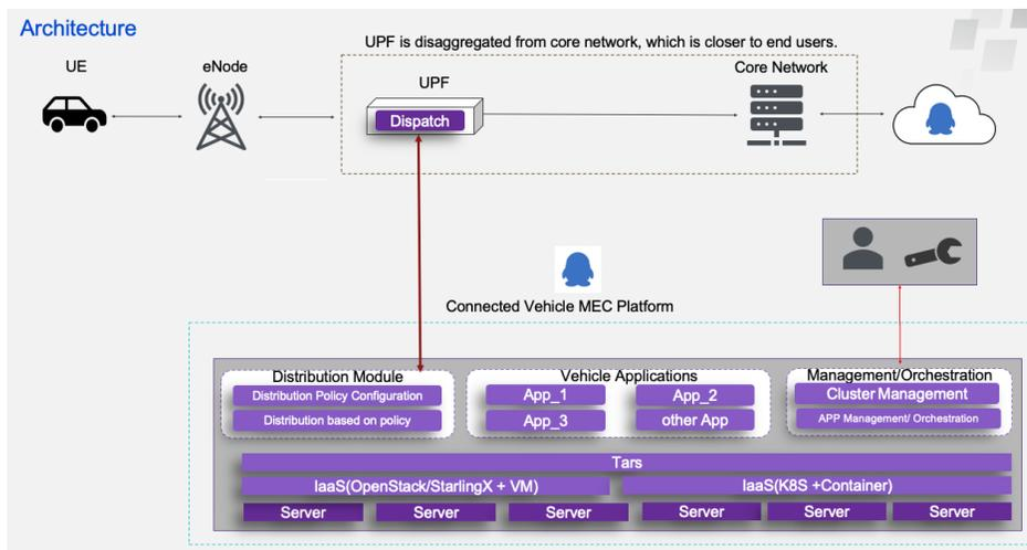
The combination of Commodity Hardware and IaaS Software provides flexible deployments, like Bare Metal, Virtual Machine as well as Container.
