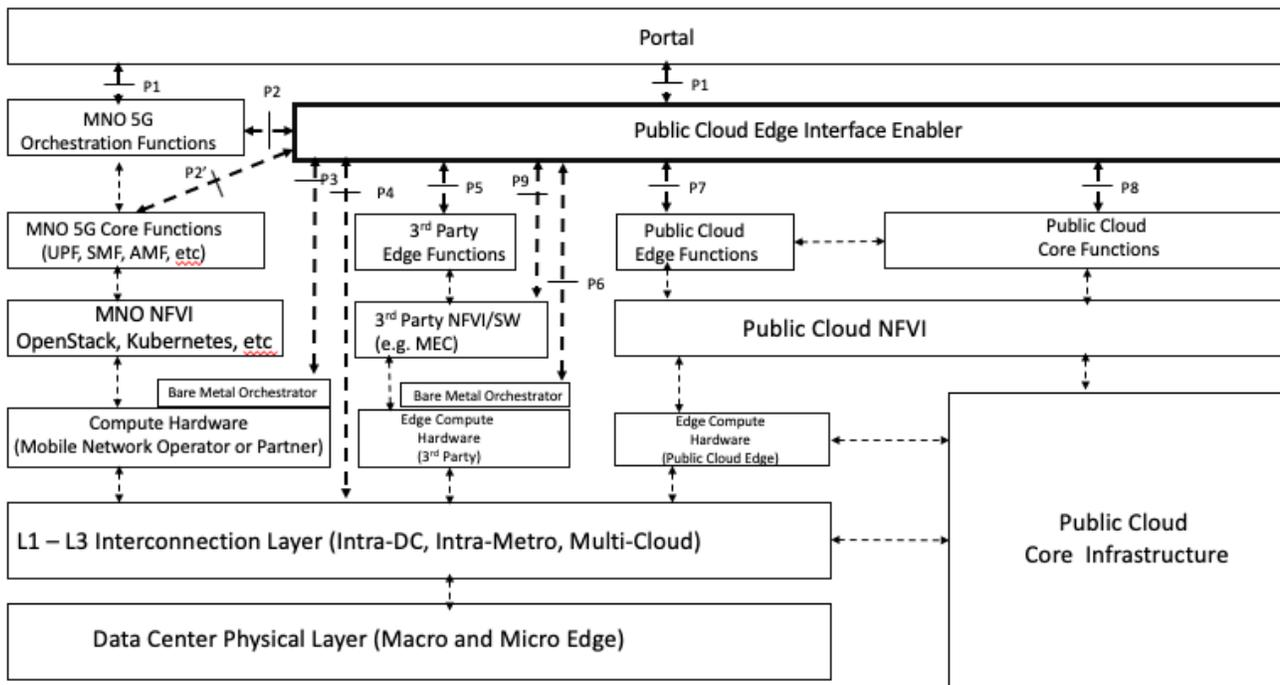
Figure 3b. The PCEI Detailed Reference Architecture.
