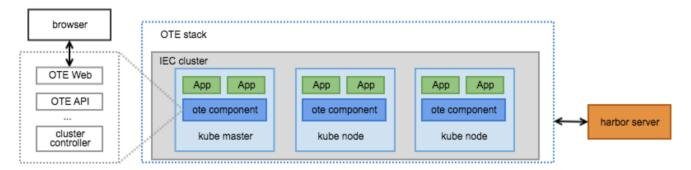
In this test scenarios, a face recognition application will be deploy to the IEC cluster via browser. The app is a server that detects the face in an image sent by client and outputs the position of objects. The usage of the server is shown in Step 4.
