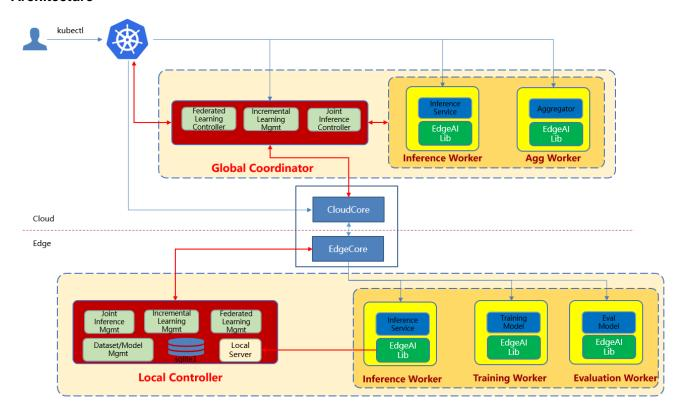
• GlobalCoordinator: implements the Edge AI features controllers based on the k8s operator pattern
