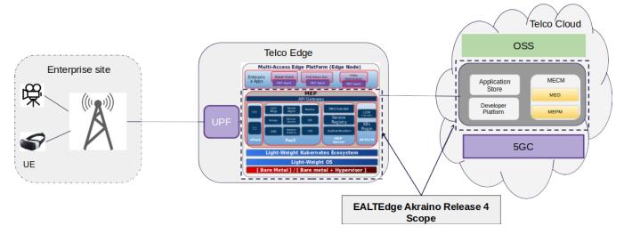
The edge computing platform(s) (MEP) needs to be installed at the telco edge(s) and Application development/management related components (MECM (MEO+MEPM), AppStore, Developer Platform) needs to be installed in Telco's cloud (private/public). Edge computing platform (MEP) provides a platform as a service environment for running "Enterprise Applications"
