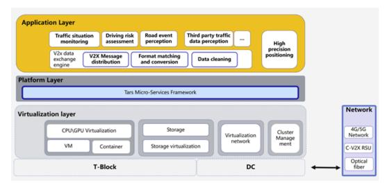
Connected Vehicle Applications include roadside traffic situation monitoring, driving risk assessment, road event perception, high percision positioning, and so on.
