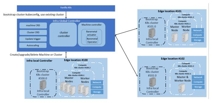
Each edge location has infra local controller, which has a bootstrap cluster, which has all the components required to boot up the compute cluster.
