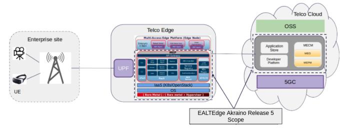
The edge computing platform(s) (MEP) needs to be installed at the telco edge(s) and Application development/management related components (MECM (MEO+MEPM), AppStore, Developer Platform) needs to be installed in Telco's cloud (private/public). Edge computing platform (MEP) provides a platform as a service environment for running "Enterprise Applications"
