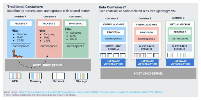
Kata Containers provides additional workload isolation with minimal performance cost. It provides default Kernel and guest image, which are highly optimized to minimize boot-time and memory footprint.
