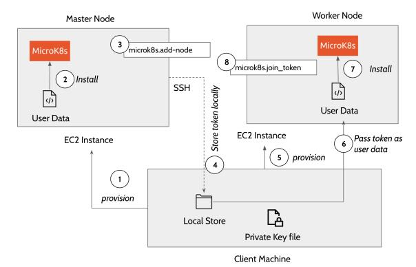
• Provision master node. The template executes EC2 user\_data on the master node that uses snap package manager to install microk8s.
