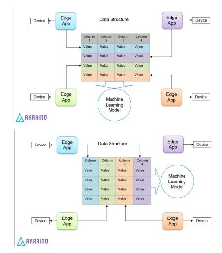
Applications group data from edges based on security methods; but data privacy is still managed by the Federated Machine Learning framework. Data, as an input of a ML model, is in a central site, and exchange of data occurs after ML processes are done. Required data gets sent back to the edge for its next process.
