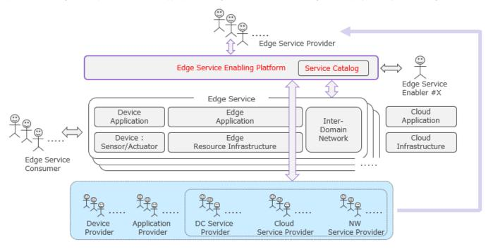
The diagram below shows how edge service catalogs encapsulate the specialized knowledge of various device, application, and service providers into a package which can be deployed in the field with minimal configuration. This benefits both the person deploying the service, by reducing the cost and effort required to design and deploy the service, and the device and infrastructure suppliers, who will see greater use of their devices and infrastructure because of the reduced friction in using them.
